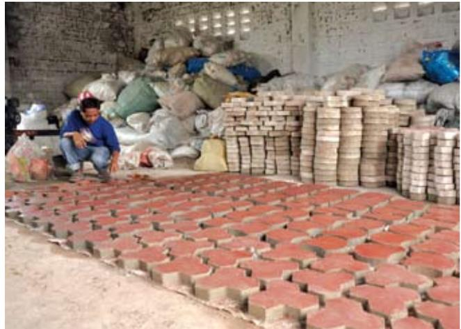
Pavers made from concrete and recovered plastic are used to improve walkways in the city. (photo: Anne Larracas)
